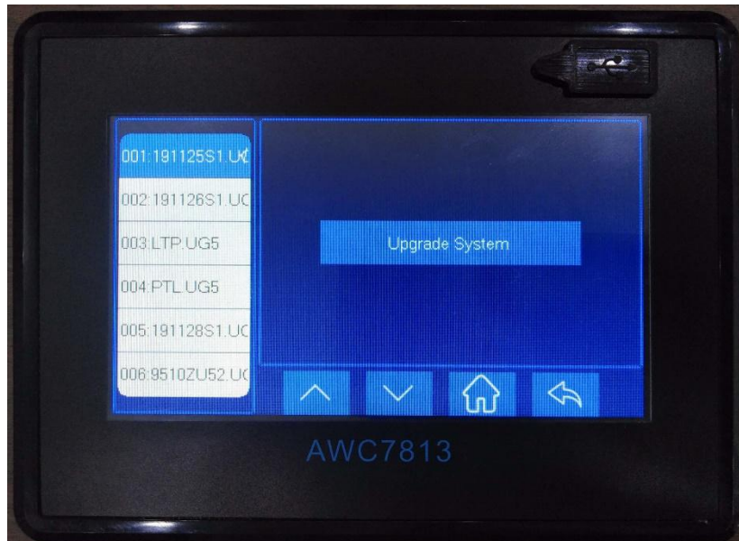
Figure3-12-2 Upgrade the mainboard
