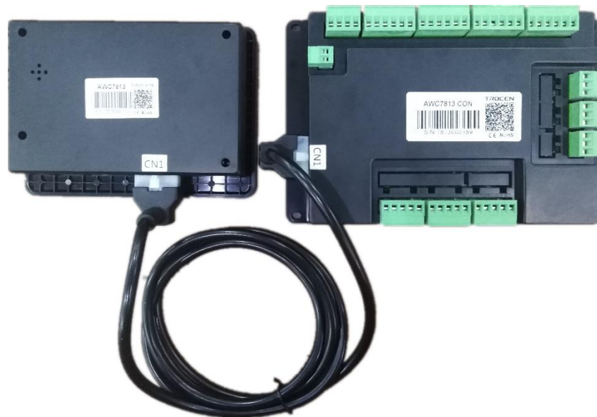
Figure 2-3-4 Connection port of panel and wiring board
