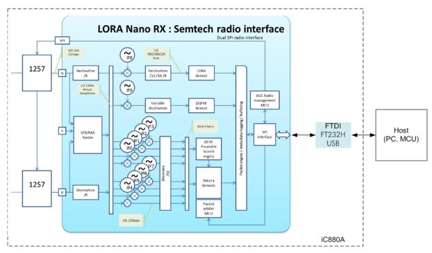
Figure 3-3: Detailed Block Diagram of SX1301 taken from [3]
