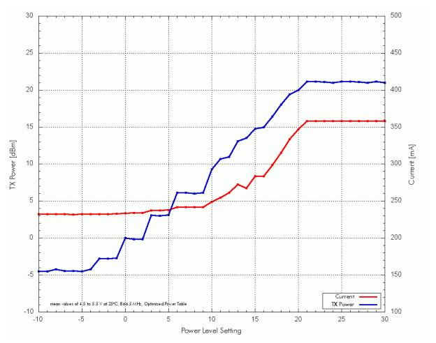
Figure 5-1: RF output power level and current consumption for an optimized configuration
