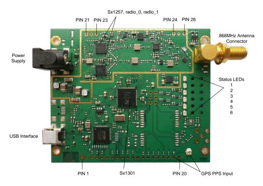
Figure 6-1: Pinout and interfaces of iC880A-USB
