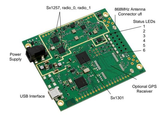
Figure 3-1: Component Overview iC880A-USB
